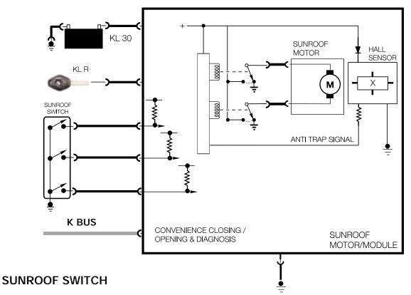
Mounted in the sunroof motor trim cover is the sunroof switch. Also similar to previous systems, the switch provides coded ground signals for system operation.
